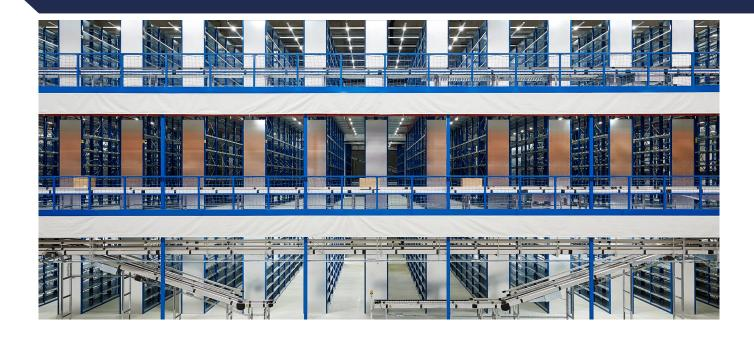
Both the components and the complete structures of NEDCON mezzanine floors are extensively tested for, among other things, load bearing capacity and safety, and more than satisfy all standards and requirements applicable in Europe and individual countries. The standard floors can hold loads of 500kg/m<sup>2</sup>, but NEDCON can also supply floors capable of dealing with loads of 1500kg/m<sup>2</sup> and more. And depending on the floor you choose, spans of 10 metres are easily achievable.
